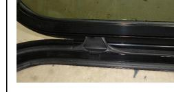
2 Remove residue adhesive with alcohol
