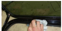
3 Apply 3M primer to surface in preparation for new seal C5-55-6074
